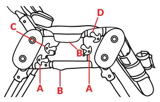
**Seat Height** - Raise or lower the legs by turning either of the four lower red levers (A).
