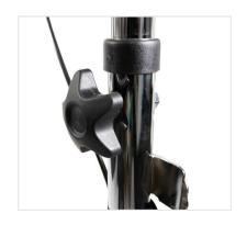
Adjust the handle height by pulling up/down on the steering column to the desired height, insert the black star bolt through the aligned holes and turn clockwise until tightened.
