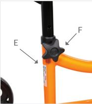
Insert the knee platform post (**D**) into the receiver tube (**E**) and adjust by pulling up/down on the post to the desired height, reinsert star bolt (**F**) through aligned holes and turn clockwise until tightened
