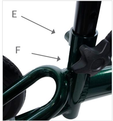
Insert the knee platform post (D) into the receiver tube (E) and adjust by pulling up/down on the post to the desired height, reinsert star bolt (F) through aligned holes and turn clockwise until tightened.
